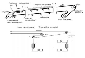
Fig. 3. Structure of belt conveyor [1]
